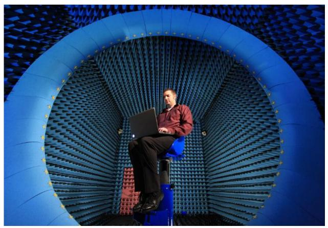
Microwave Vision test facility to test devices while in use - an exclusive Microwave Vision system which allows engineers to test devices in close-to-real situations.
