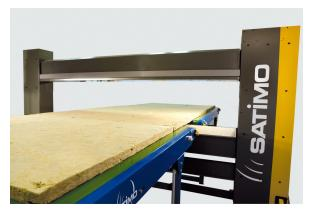
**Dentro LRX** makes it possible to have permanent quality control on a continuous production line, by immediately detecting defects in any sort of non-metallic material.
