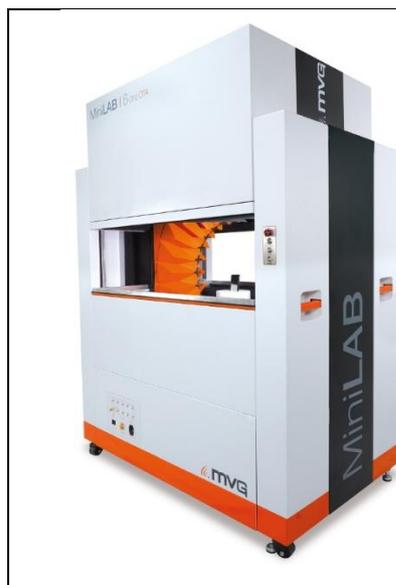
The **MiniLAB I 6 GHz OTA** uses proven electronic scanning technology to evaluate the electromagnetic field on a full sphere surrounding the antenna. Power is measured using an array of bipolar probes that scan the object within a few seconds.
