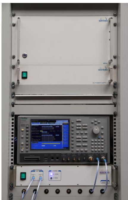
Anritsu MT8820C in SATIMO's measurement rack
