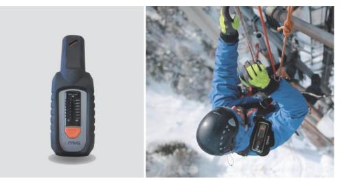
Significant sales of EME Guard XS devices have been achieved since its launch in 2014, with future orders in the pipeline. EME Guard XS is a 'must-have' RF Safety tool; an EMF monitoring device which alerts all personnel operating near antennas to excessive exposure to RF levels.
